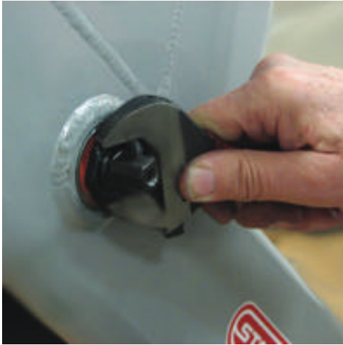
Tighten the nut to 30 lbs-ft
