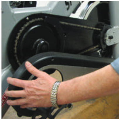
Tighten the nut to 30 lbs-ft
