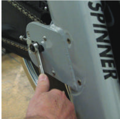
Tighten the nut to 30 lbs-ft
