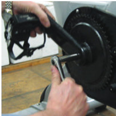
Tighten the nut to 30 lbs-ft
