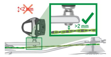
**9** If the pedal rubs the chain, add one washer (included) between the spindle and the crank arm to increase clearance.
