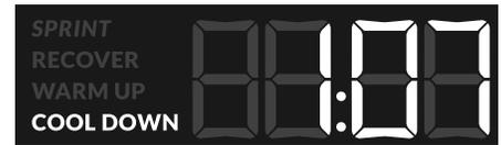
If a workout is completed and the user continues to use the machine, Cool Down will automatically start. The Console will track the time in Cool Down, and display the workout results of the completed workout. Cool Down values are not added to the results or saved. Cool Down is ended with a push of the PAUSE/STOP button or no RPM for 10 seconds.
