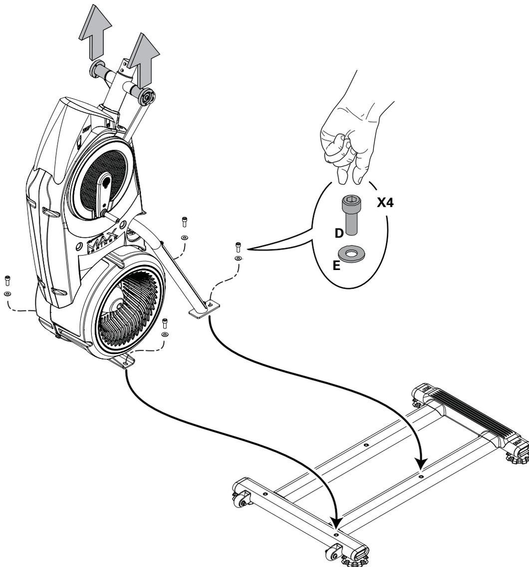
4. Attach Stabilizer Shroud to the Frame Assembly
