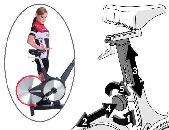
Figure 10. Seat Height Adjustment
